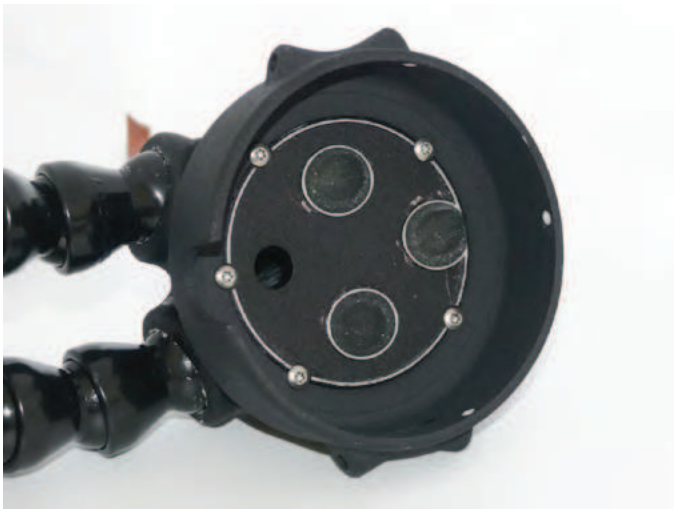
Inside the head of the snoot, showing the three pick-up cores
